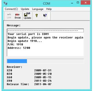
4. After the processing completes, please close the uploader, and then power off and power on the receiver again.
